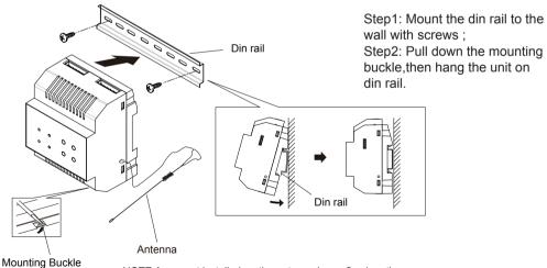
NOTE:A magnet installed on the antenna base, fixed on the wall directly adsorbed iron (iron Fortunately, pre-installed on the wall) place. In addition, the antenna should be installed in the open place, there should be no obstructions around.
