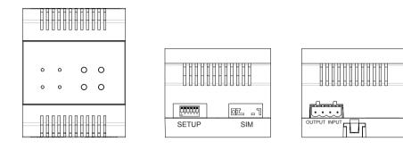
SETUP: SIM: Output: Input: DIP switches. SIM card slot. Output port,connect to Monitor. Input port,connect to power supply.
